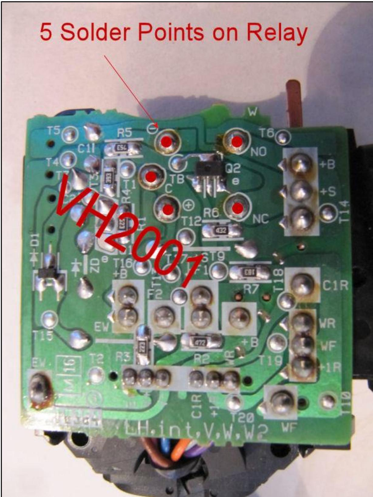
Use a desoldering tool (under \$10 here [Amazon Desoldering Tool](#))...
